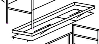
WITH PLATFORM ON TOP RUNG IT GIVES A WORK LEVEL OF LESS THAN 2M.
